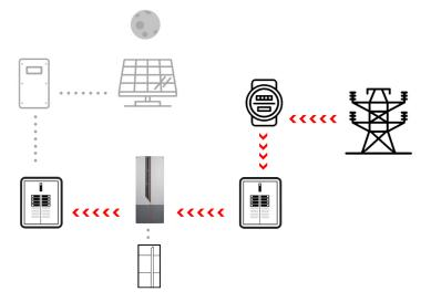
Figure 3 – GDI Power Flow without PV
