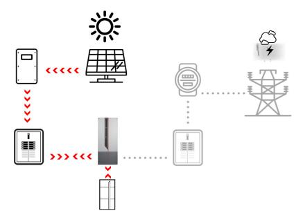
Figure 2 – GDI Power Flow with Active PV
