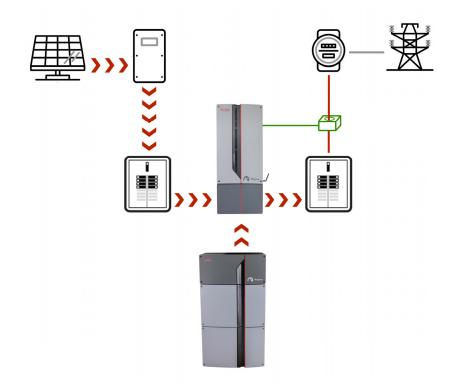
Figure 8 – ToU Power Flow with Current Transducers
